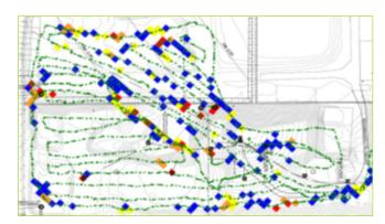
Based on a screening with a handheld FID detector, a site plan is developed with color codes showing where and relatively how much methane is emitted.
