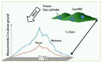
The total emission of methane is calculated based on the ratio of methane and tracers measured in a trench downstream from the landfill.
